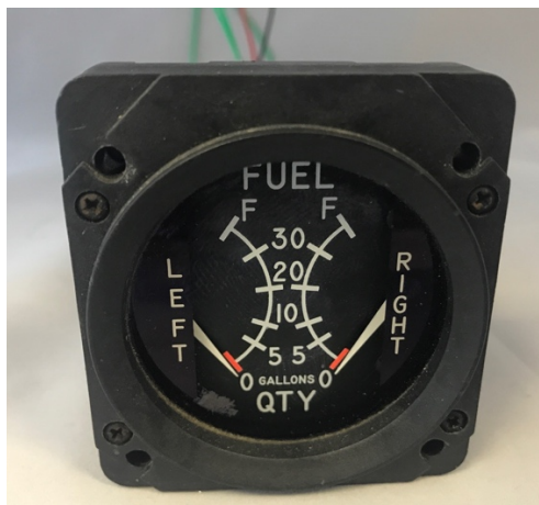
Figure 6-2 Rochester Fuel Gage
