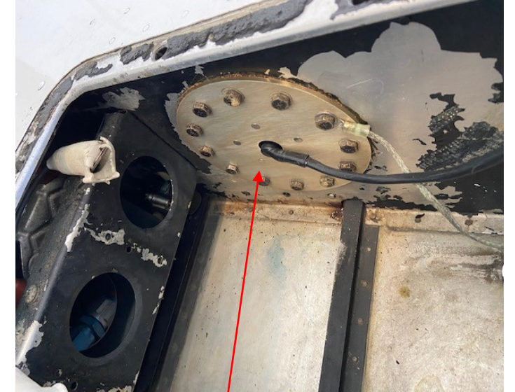
CiES Fuel sender and bracket installed
